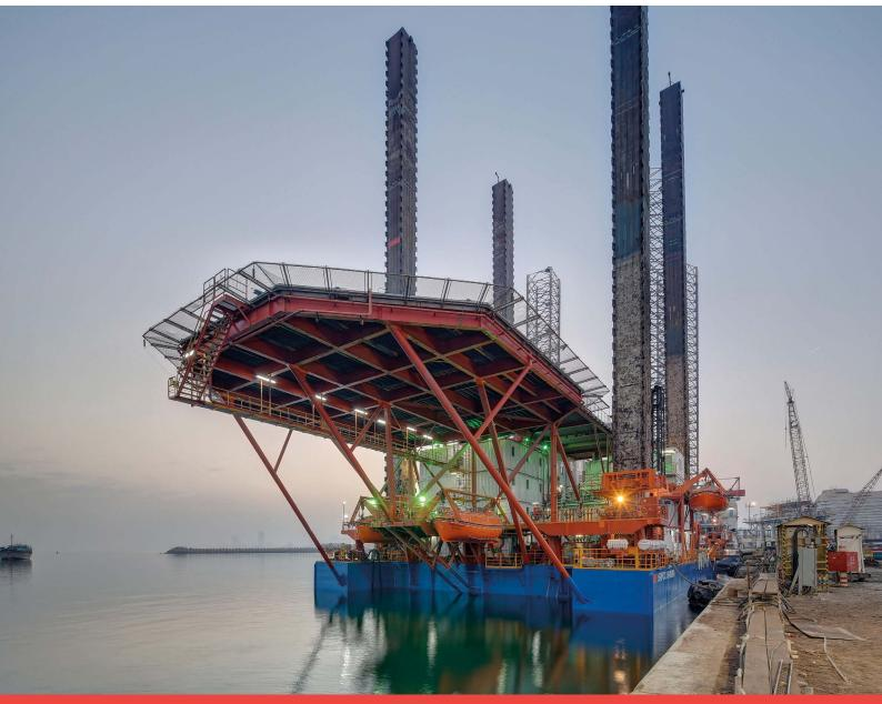
MAIN CRANE CAPACITY 22.7 t | ACCOMMODATION 220 POB | MAX WATER DEPTH 46 m | DECK SPACE 355 m<sup>2</sup>
